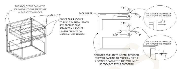
\* REFER TO <u>FG-2</u> & <u>FG-2.5</u> (SEE "WORKSHOP" SECTION) FOR FG PROFILES & "THE COLLECTION" FOR MATERIAL LENGTH. ALSO REFER TO <u>FINGER GRIP INFORMATION</u> (SEE "BASE CABINETS" SECTION)
