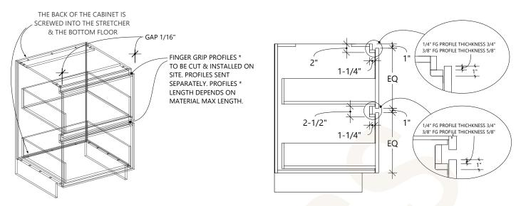
\* REFER TO <u>FG-2</u> & <u>FG-2.5</u> (SEE "WORKSHOP" SECTION) FOR FG PROFILES & "THE COLLECTION" FOR MATERIAL LENGTH. ALSO REFER TO <u>FINGER GRIP INFORMATION</u> (SEE "BASE CABINETS" SECTION)
