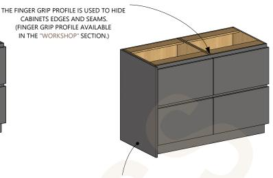
A PANEL CAN ALSO BE USED TO CREATE A FINISHED END.
